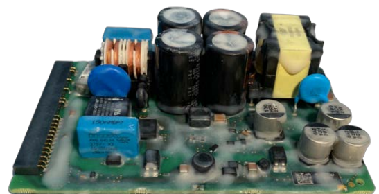
Figure 2: The PCB used for evaluating the process is conformal coated with the new material according to the coverage plan.
