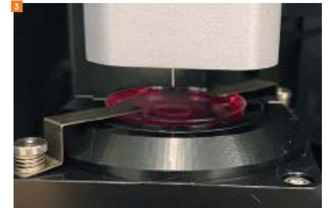
3 The mechanical properties of the cornea measured using instrumented indentation.
