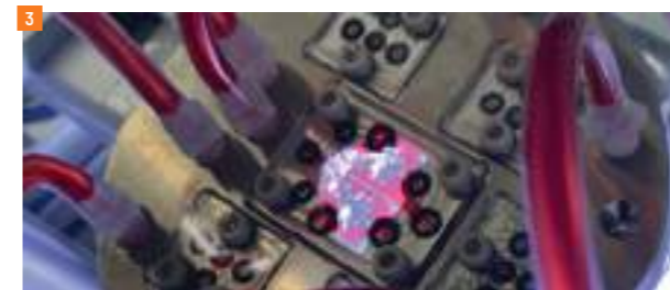
Microfluidic chip to model the blood flow in the heart muscle.
