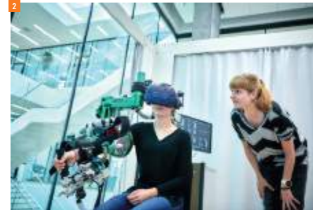
Robotic motor training with ARMin exoskeleton in immersive virtual reality
