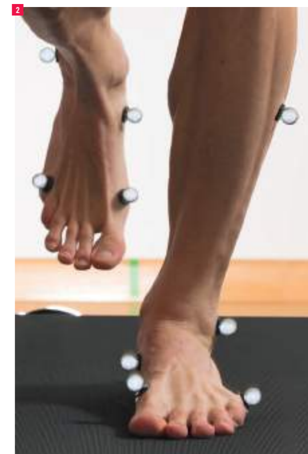
Clinically oriented measurement of foot kinematics by quantifying navicular bone motion using four reflective markers and 3D motion capture
