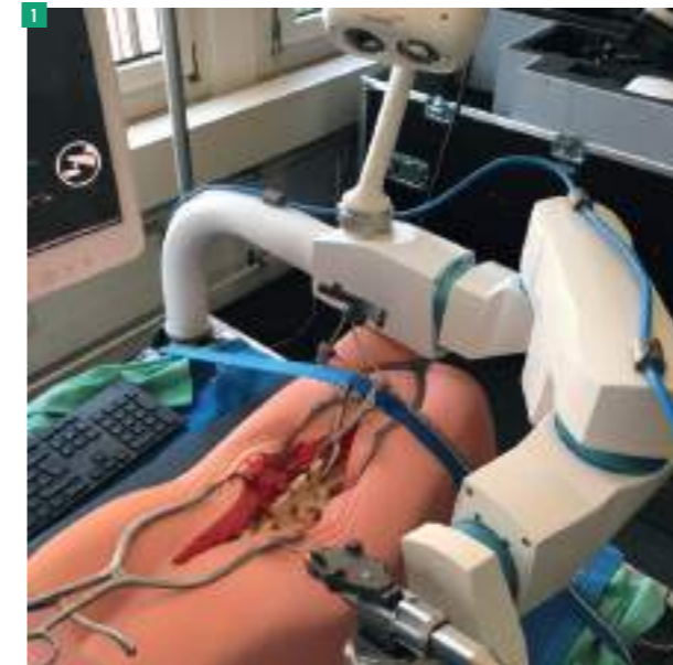
Laboratory set-up of spine model and robotic arm with attached high-speed drill for high-precision drilling through the pedicle of the targeted vertebral body.
