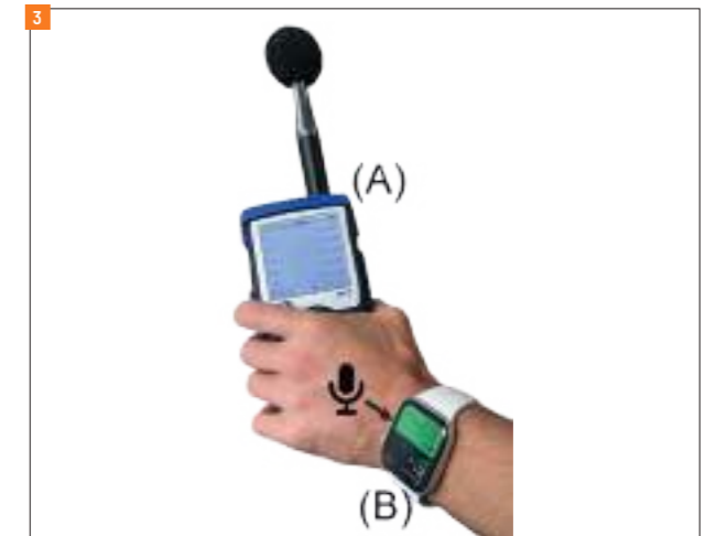
Noise monitoring using a sound level meter (A) and a smartwatch (B).
