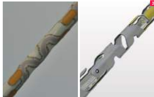
3D CAD design of a smart catheter with active transducers embedded (left) and prototype of a smart catheter with FEM-optimized LCP design for multiple passive electrodes
