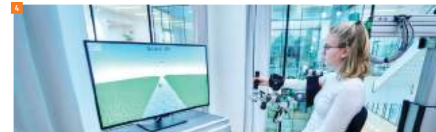
Virtual inverted pendulum task with ARMin exoskeleton robot
