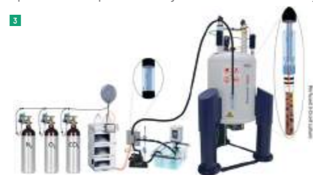
Bioreactor for online Metabolomics of living cells inside the NMR.
