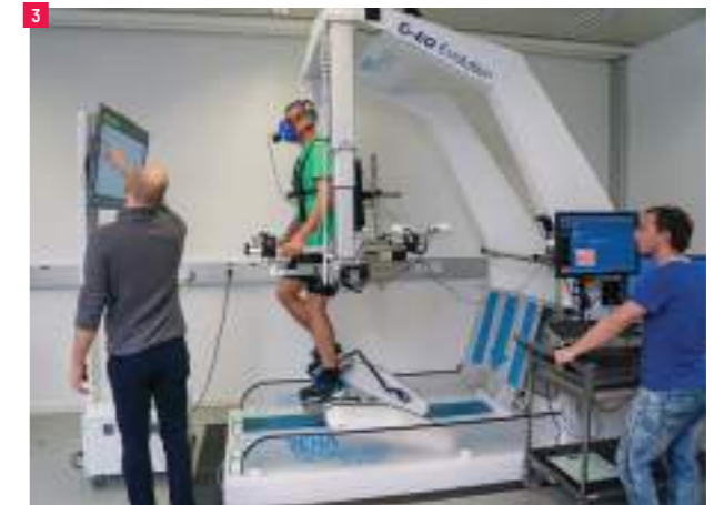
Cardiopulmonary rehabilitation with the G-EO System end-effector gait-rehabilitation robot
