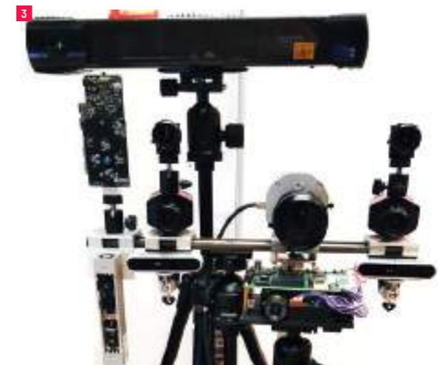
Test setup of different 3D measurement technologies and devices for the measurement of the human back
