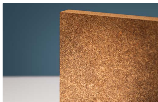
Figure 1: Cocoboard: a medium density fibreboard made of coconut husk and tannin-based adhesive
