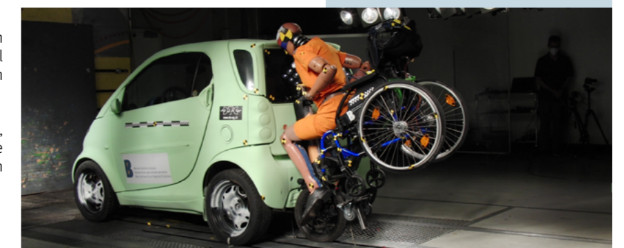
▼ Figure 4 – Crash test at 20km/h: collision with the rear of a stationary vehicle.
