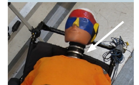
▲ Figure 3 – Final position of the crash test dummy, after impact, on a wheelchair with no headrest.
