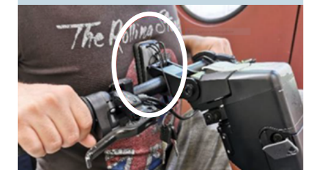
▲ Figure 2 – Display screen on the E-Pilot handlebars can come into contact with the chest on impact.
