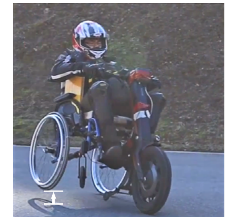
▲ Figure 1 – Lifting of rear wheel following excessive transverse acceleration.
