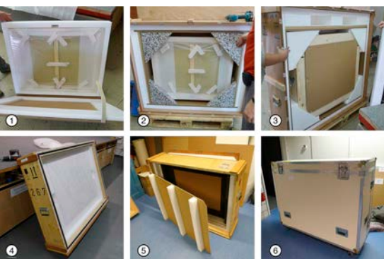
Figure 1 Packing systems tested: (1) cardboard box, (2)–(5) insulated boxes, (6) flight case. Descriptions are listed in Table 1
